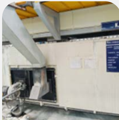
At KOD (To remove dirt and grease from component)
